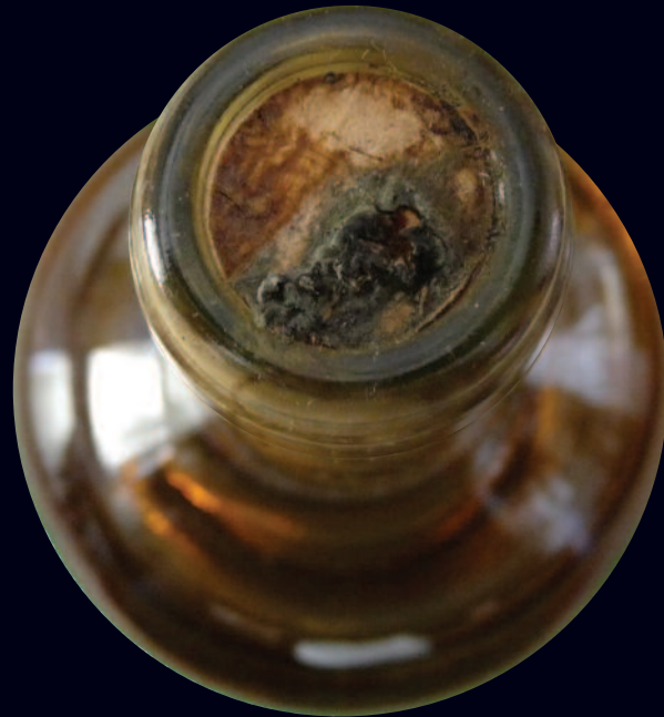
Example of wine seepage on the outer surface of a cork
