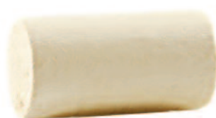
one-piece colmated natural cork stopper treated using cork dust and glue to eliminate surface defects
